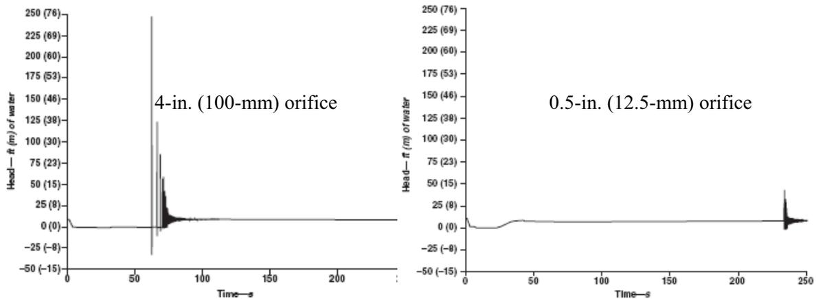
Figure 12: Surge analyses for secondary pressure surges due to final air release through 4 inch and 0.5 inch air discharge orifices<sup>9</sup>
