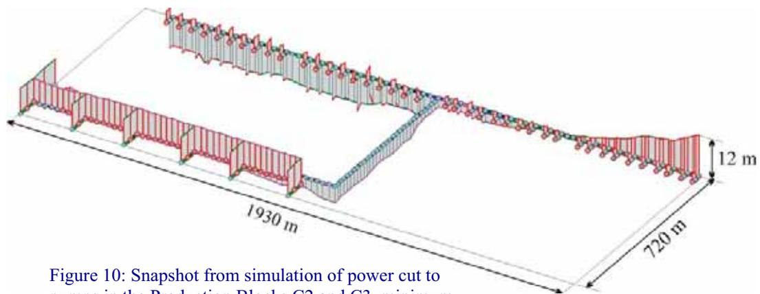
Figure 10: Snapshot from simulation of power cut to pumps in the Production Blocks C2 and C3, minimum pressures with vaporous cavitation<sup>10</sup>
