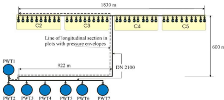
Figure 7: Layout of the system and presentation in the model<sup>10</sup>
