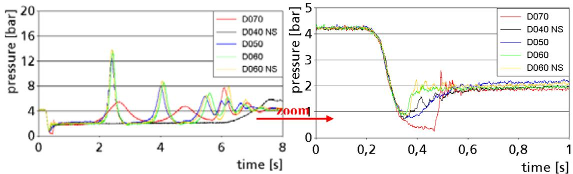
Figure 18: Comparison of pressure histories down-stream from the shut-off valve when different types of air valves are active at both PO 3 and PO 9 at the same time. The air valves at PO 3 and PO 4 are of the same type and size <sup>6</sup>
