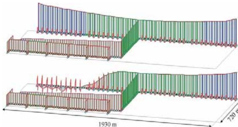
Figure 9: Snapshots of simulation of power cut to pumps in the Production Block C2 with vacuum breakers, steady state (upper) and minimum pressures (lower) <sup>10</sup>
