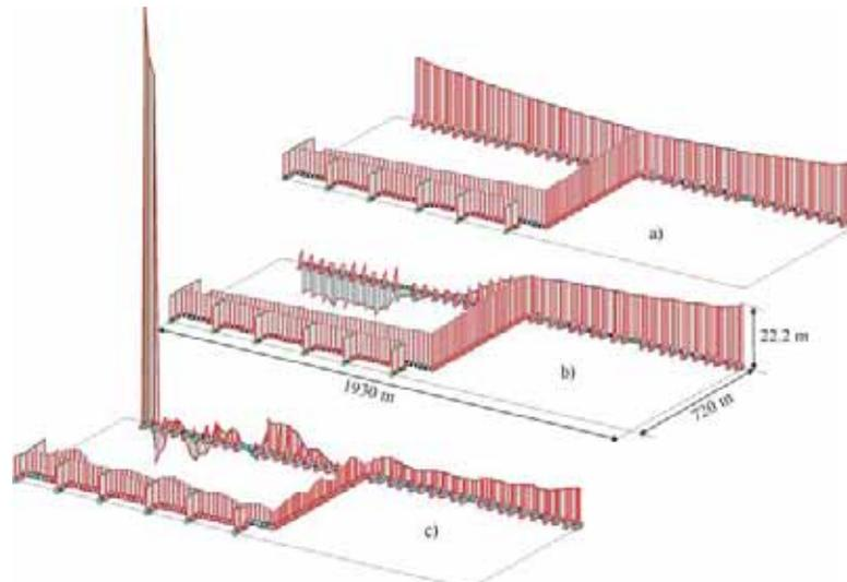
Figure 8: Snapshots from the simulation of power cut to pumps in the Production Block C2, a) steady state, b) minimum pressures with vaporous cavitation, and c) maximum pressures after cavity collapse <sup>10</sup>
