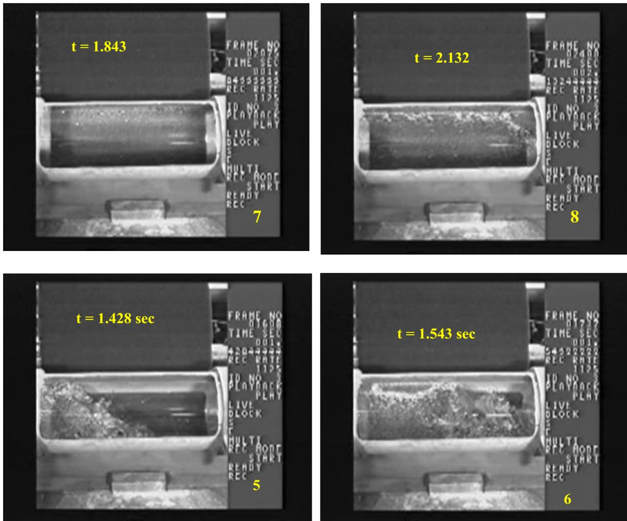
Figure 15: Views through a window, into the pipeline of the Fraunhofer UMSICHT surge test rig, showing water column separation and return and vapor cavity formation and collapse, down-stream from a fast closing shut-off valve. These views are frames from a video that was filmed at 1125 frames per second to capture the event and process. <sup>24</sup>
