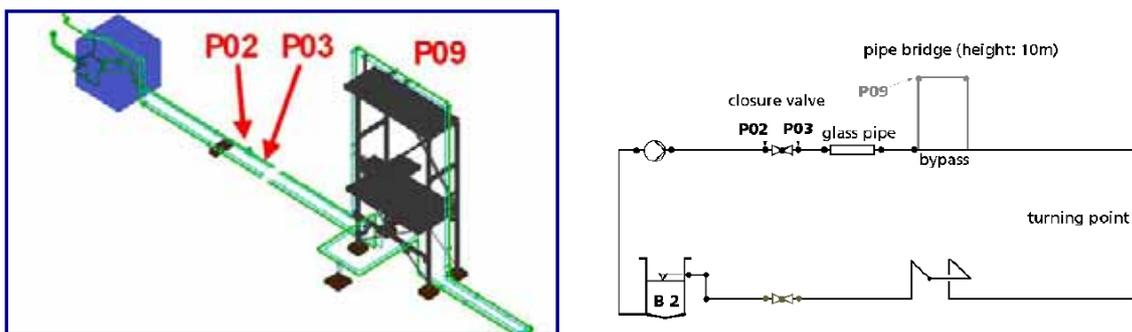
Figure 14: Faunhofer UMSICHT Division of Pipeline Technology surge test rig <sup>6/22</sup>
