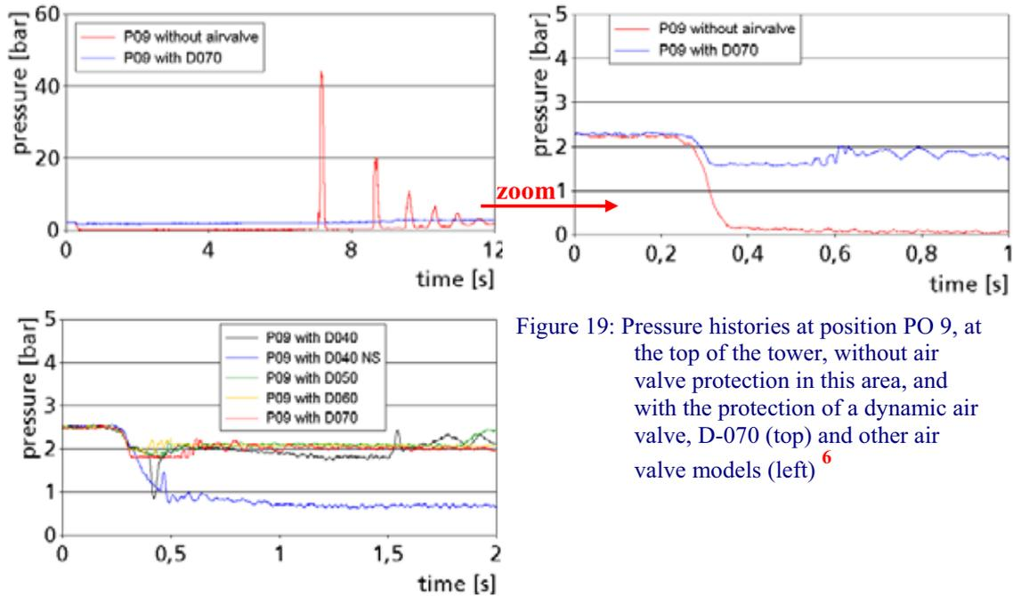
Figure 19: Pressure histories at position PO 9, at the top of the tower, without air valve protection in this area, and with the protection of a dynamic air valve, D-070 (top) and other air valve models (left) <sup>6</sup>
