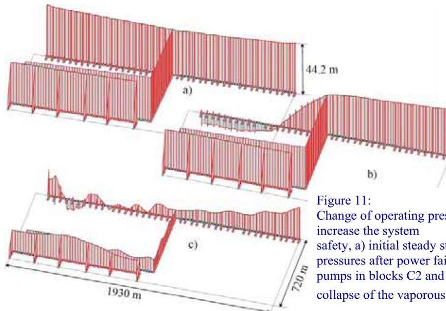
Figure 11: Change of operating pressure as a measure to increase the system safety, a) initial steady state, b) minimum pressures after power failure for pumps in blocks C2 and C3, c) moment after collapse of the vaporous cavity.<sup>10</sup>
