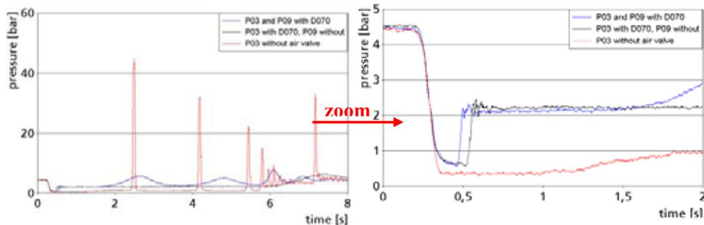
Figure 16: Graphs of pressure histories down-stream from the shut-off valve: red line, no air valve protection; black line, only the air valve at PO 3, down-stream from the shut-off valve, is active; blue line, both air valves, at PO 3 and at PO 9, at the top of the tower, are active. Dynamic D-070 air valves in both locations <sup>6</sup>
