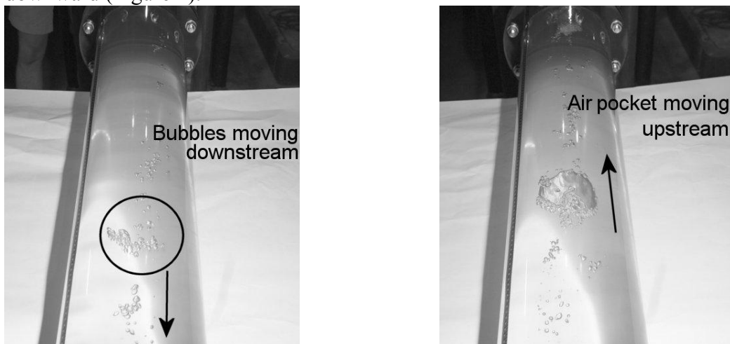
Figure 3. Left: Small bubbles moving downstream, Right: Air pocket moving upstream.
