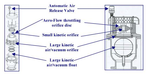
A.R.I. D-060 HF NS high- flow, non-slam, combination air valve
