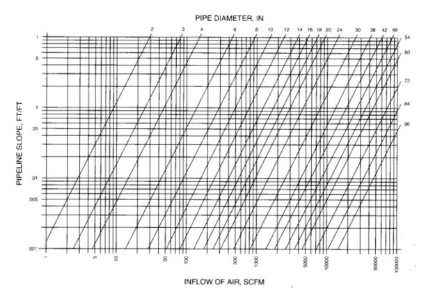
Kinetic Large Orifice Air Intake Requirements According to AWWW Manual M51
