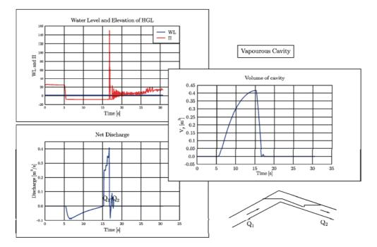
System behavior at the most upstream cavity, after power cut to pumps in PB C2
