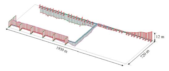
Pressure envelope snapshot from simulation of power cut to pumps at PB C2 and PB C3, at minimum pressures with vaporous cavitation
