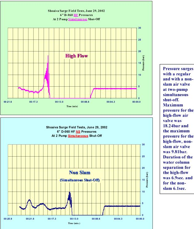
and with a nonslam air valve at two-pump simultaneous shut-off. Maximum pressure for the high-flow air valve was 18.24bar and the maximum pressure for the high-flow, nonslam air valve was 9.81bar. **Duration of the** water column separation for the high-flow was 6.9sec. and for the nonslam 6.1sec.
