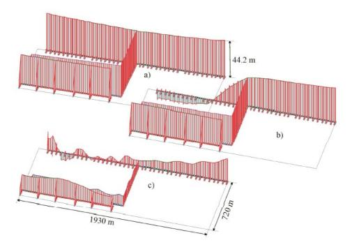
Pressure envelope snapshots of simulation of power cut to pumps at C2 and C3, with vacuum breakers every second pump connection: a) Steady state, b) minimum pressure after power cut, and c) moments after collapse of the vaporous cavity.
