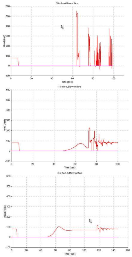
Here, also, the difference in the pressure surges due to "Air Slam" are very significant, as can be seen in the graphs below.
