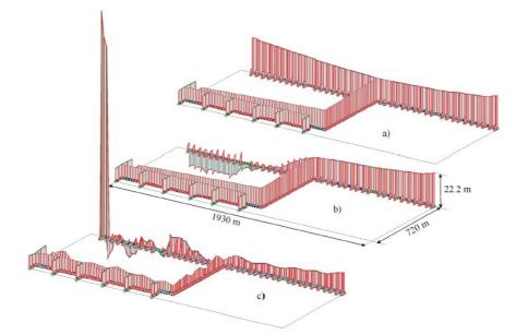
Ivetić's pressure envelope snapshots of the first simulation: a) Steady State, b) Minimum pressure with vaporous cavitation, and c) maximum pressure at cavity collapse
