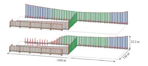
Pressure envelope snapshots of simulation of power cut to pumps at PB C2 with vacuum breakers at every second pump connection. Steady state, above, and minimum pressures, at bottom
