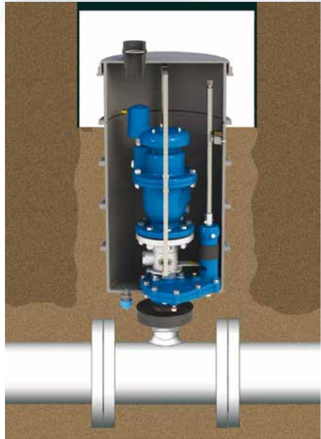
Prior to site preparation and installation, please refer to the D-060-C HF SB Installation and Maintenance Manual for all the relevant instructions and information. The manual can be obtained by contacting the A.R.I marketing dept. or downloading the file from our website.
