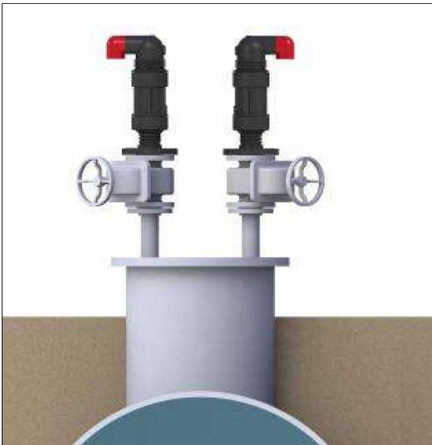
Two Air Valves on an Air Trap with separate Isolating Valves. Air Valve outlets face outward and the Isolating Valves at 45° to Air Valve outlets
